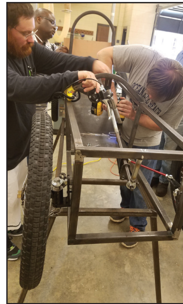
The Indy race followed a 10-week period of intense, collaborative work by VGCC students to design, procure parts, manufacture parts and construct the car. At left, VGCC Welding Technology students fabricate the frame of the car, based on a basic layout designed by Mechatronics Engineering Technology students. At right, Mechatronics Engineering Technology students work to complete the construction on the electric car.
