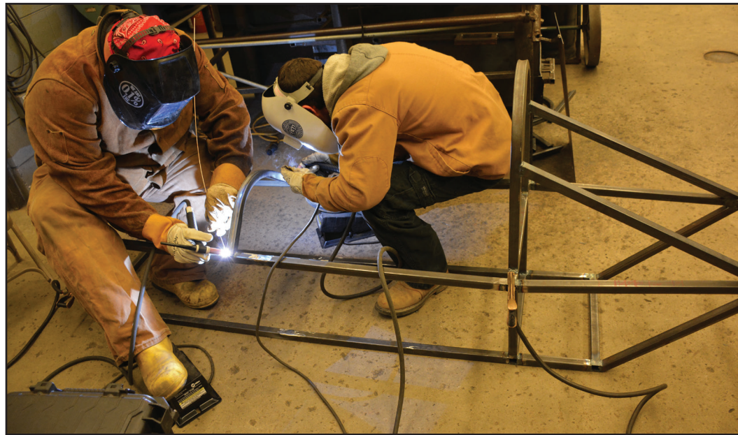
The Indy race followed a 10-week period of intense, collaborative work by VGCC students to design, procure parts, manufacture parts and construct the car. At left, VGCC Welding Technology students fabricate the frame of the car, based on a basic layout designed by Mechatronics Engineering Technology students. At right, Mechatronics Engineering Technology students work to complete the construction on the electric car.
